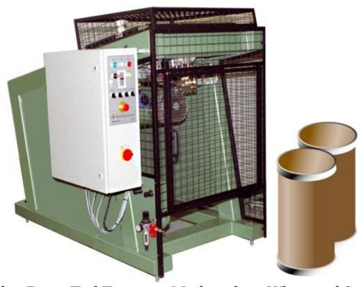
The Fibre Drum End Trimming Machine from White and Street International removes the metal rims from fibre drums. The drum body is then available for recycling, and can be flattened to a small volume for storage.
