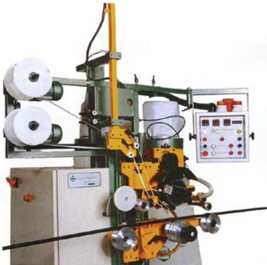
The dual driven marking foil feed system can be built to suit any size of bobbin or foil pack.
