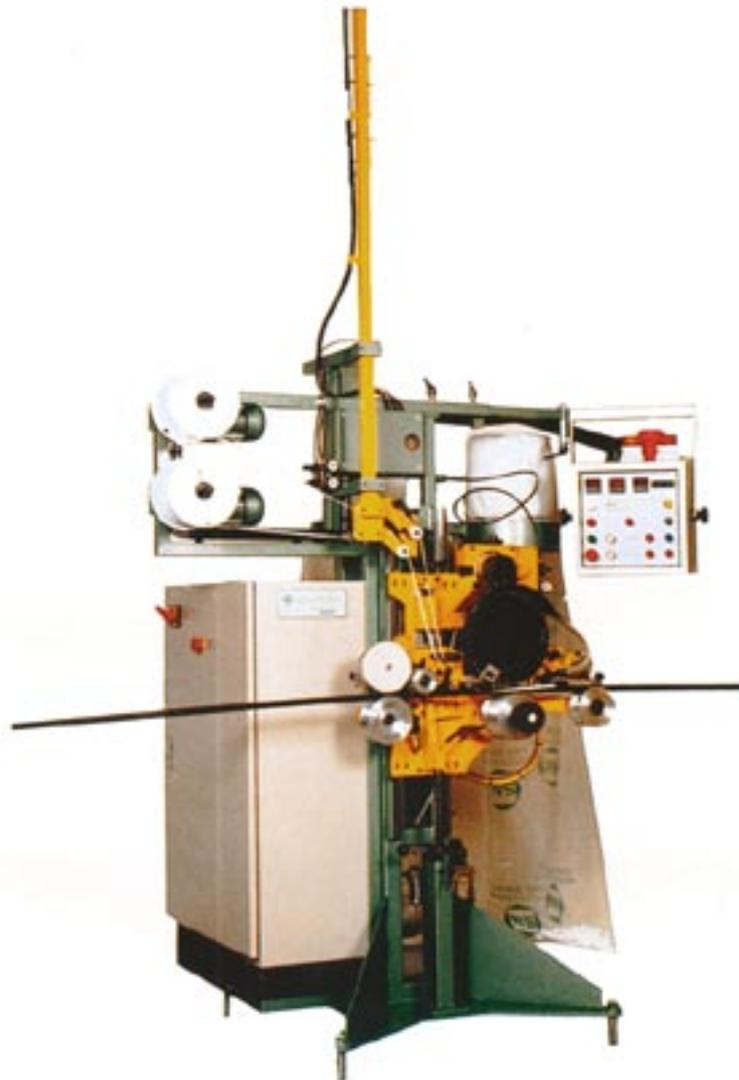
The WS933 is the third generation of servo driven cable markers, designed to print progressive measurements and legends in steps of one meter or two feet, at high speed and with extreme accuracy of print interval. Robust construction ensures rigidity, which is the first requirement of high speed marking. Marking wheels of one meter and two feet are quickly interchangeable, to minimise down time. Fine length scale adjustments can be made on the run in increments of 0.2mm (.008 inch).
