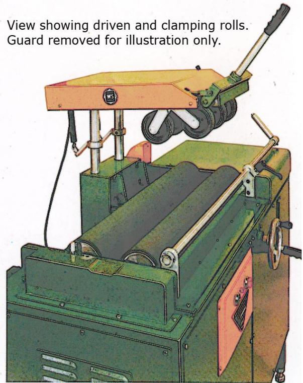
View showing driven and clamping rolls. Guard removed for illustration only.
